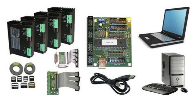
Installation of PlanetCNC CNC USB Controller requires a USB equipped PC or laptop along with motor drivers appropriate to the motors in use. The USB CNC controller is compatible with the vast majority of motor drivers that use step/direction signals.
